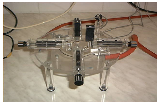
Figure 1: The uniaxial and biaxial laboratory test machines. The strain gauges were pasted on material of spring steel, the jaws were made of eloxed aluminium and the gripped points were fixed on thread slides.
