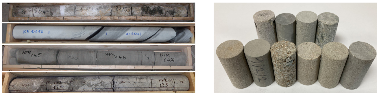
Figure 5 | TZ field core selection procedure – Geology rock drill core samples in wooden box and prepared plugs | Source: MOL Plc. (author's own pictures), 2022
