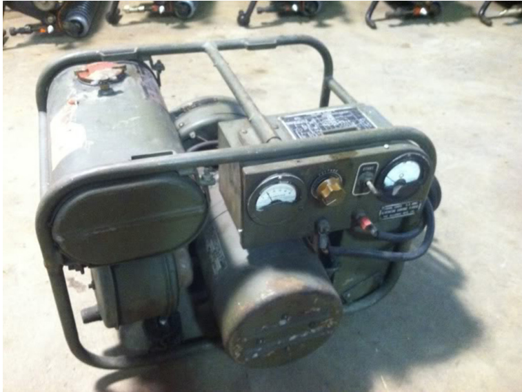
Figure 2. A typical small gasoline generator US GE-12-G from WW2. It has a 0.5 kW air-cooled 2-stroke 2-cylinder engine and produces 12 volts DC. [5: 572]
