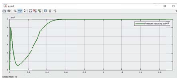
Fig. 16 Reductor pressure during simulation
