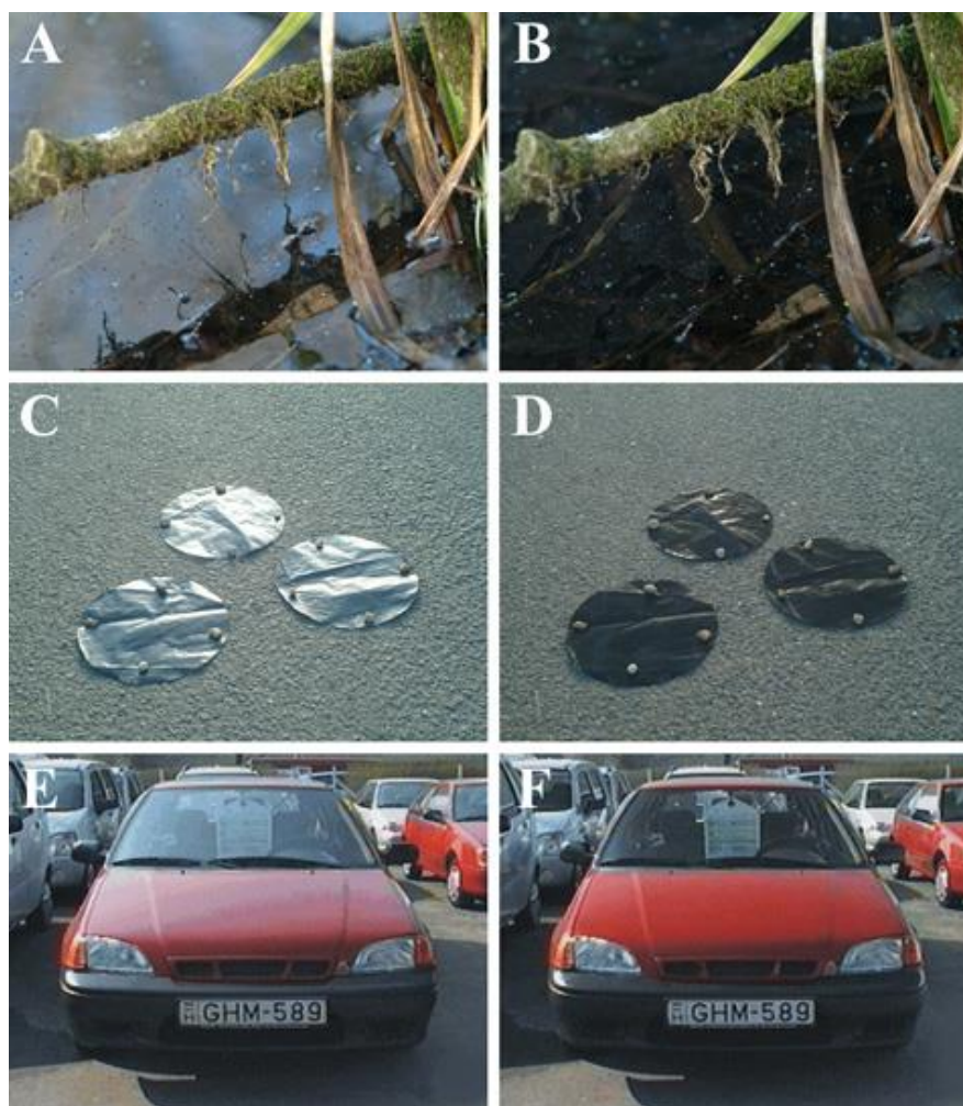
Fig. 1. Pictures on the left side (A, C, E) were taken through a linear polarizer with horizontal transmission axis, while pictures on the right side (B, D, F) were taken through a polarizer with vertical transmission axis. (A-B) Water surface. (C-D) Shiny dry black circular plastic sheets on a dry asphalt surface. (E-F) Red car (Suzuki Swift). Photographs taken by György Kriska (A-D) and Gábor Horváth (E-F)
