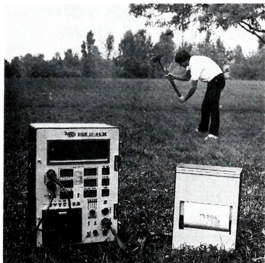
Field work with ELGI's 24 channel portable seismograph
