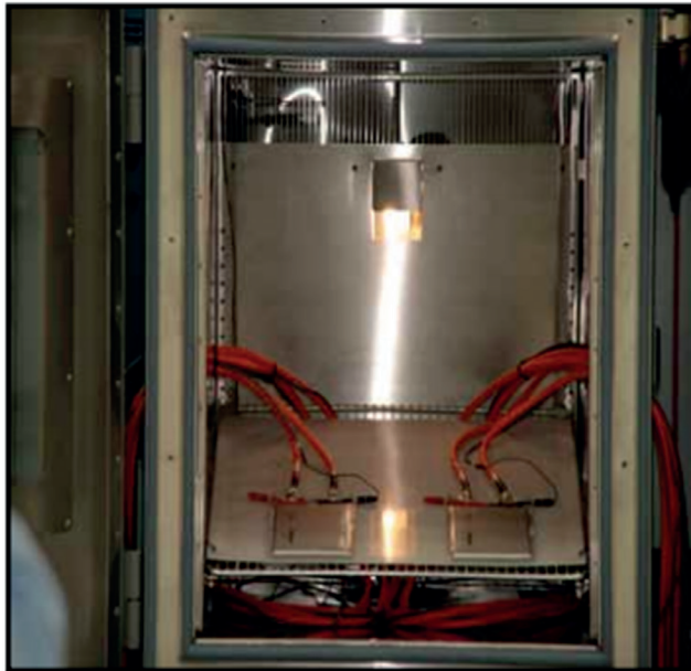
Figure 2 Battery Cell testing chamber (inside view) Source: 'Environmental Chambers.'
