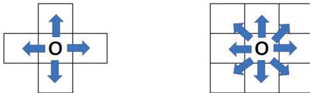
Figure 4 The two vehicle models. Left is the actual four-move; right is the possible eight-move. Source: created by the authors
