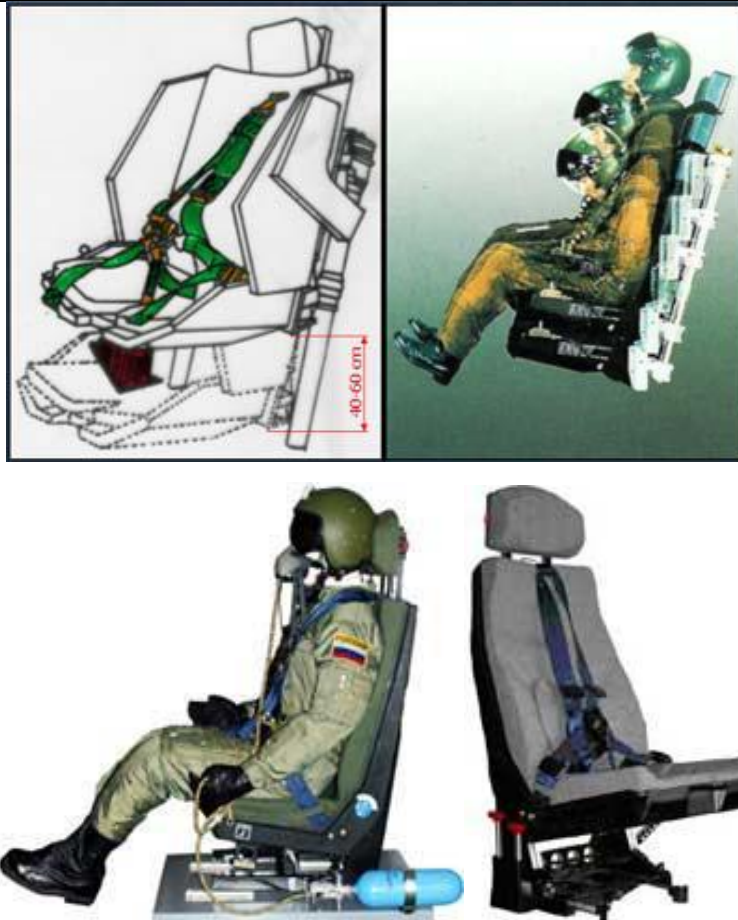
Figure 2. An AK-2000A pilot seat that absorbs impact energy, suffering a non-flexible change of form [2]
