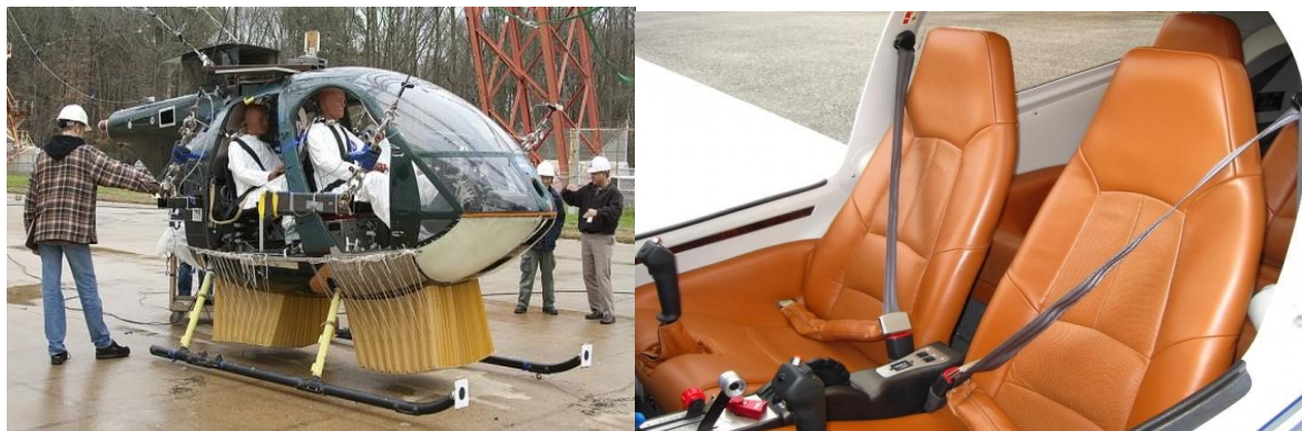
Figure 4. The airbag system fitted externally on the MD-500 and the one fitted onto the seatbelt in Da-40 [8]
