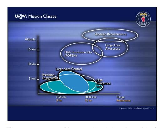
There are a great number of different tasks where UAVs could be useful, and also preferred compared to manned aircraft. The different tasks will require rather different UAV designs and different sensor equipment, Electronic Warfare (EW) equipment and weapon loads.
