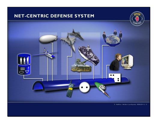
The NET-Centric System constitutes a common net in which Army, Navy and Air Force units, Command Centers etc. are tied together. The user will have the possibility to have access to all relevant information, depending on the user's role. Actually the infrastructure of the existing Internet will be used, and a virtual net created with secure access control.
