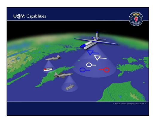
This is an example where potential intruders have been detected by a HALE, and quick reaction UAVs with high resolution sensors have been sent out to identify two ships on the sea (one ferry out of schedule, one military vessel). The symbols below the HALE represent known, unknown and hostile ships.
