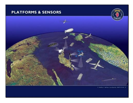
This picture illustrates different sensors and sensor platforms that can be used for surveillance over sea, in this case the Baltic.
