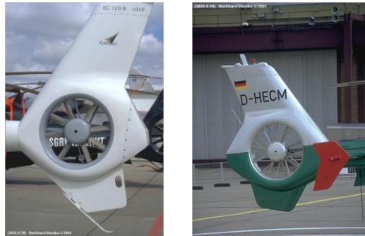
Fig. 3. Fenestron of EC-120 and EC-135 helicopters.
