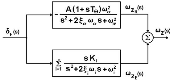
Fig. 1. The Aircraft Rigid Model and Elastic Model
