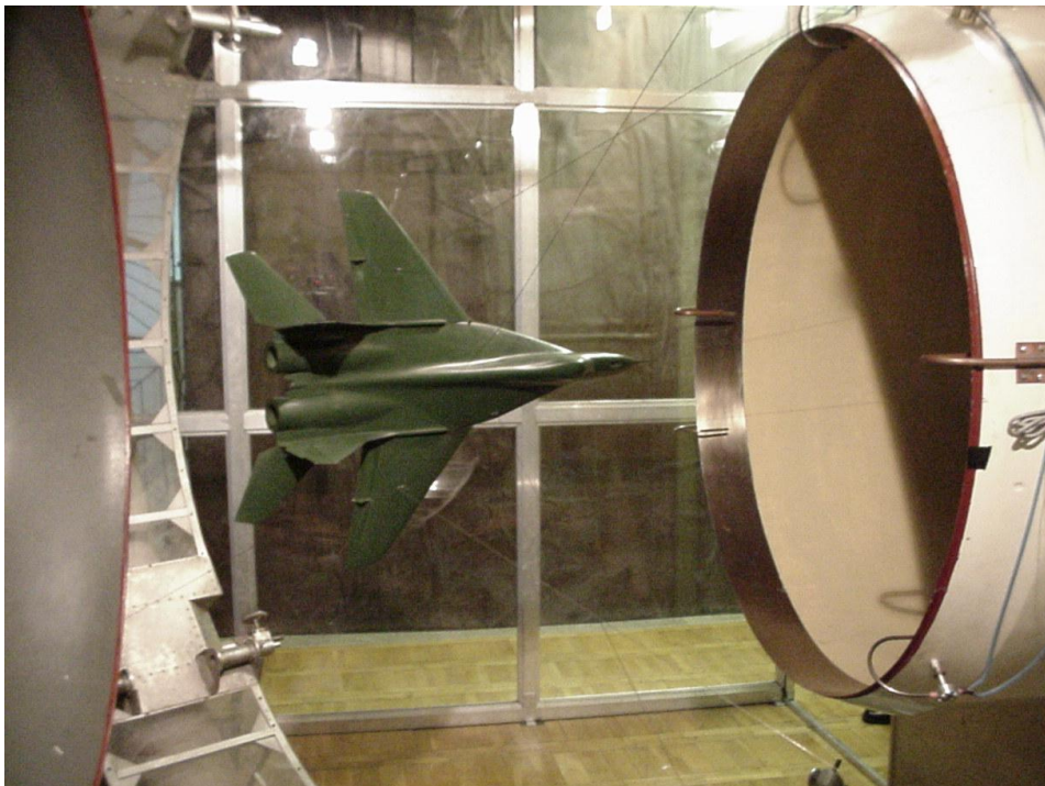
Fig. 2. The subsonic wind tunnel with capabilities of environment temperature reduction up to minus 10 centigrade.
