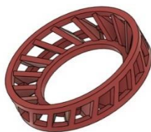
Figure 2. 3D printed spacer used in experiments
