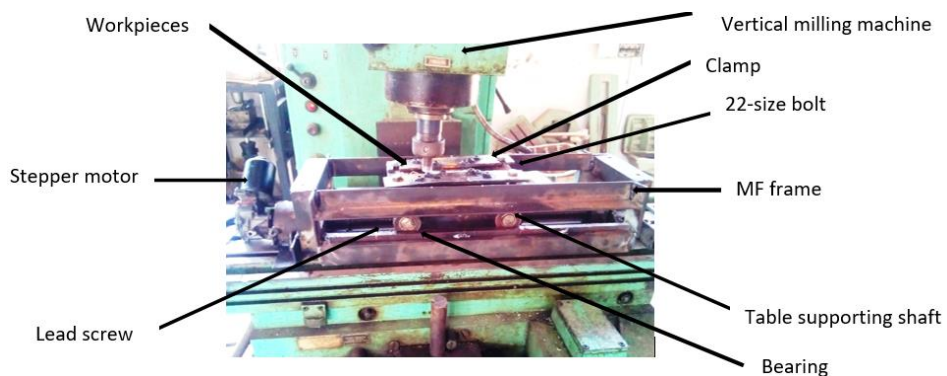
Figure 5: The developed MFS being used for FSW Operation on VMMT
