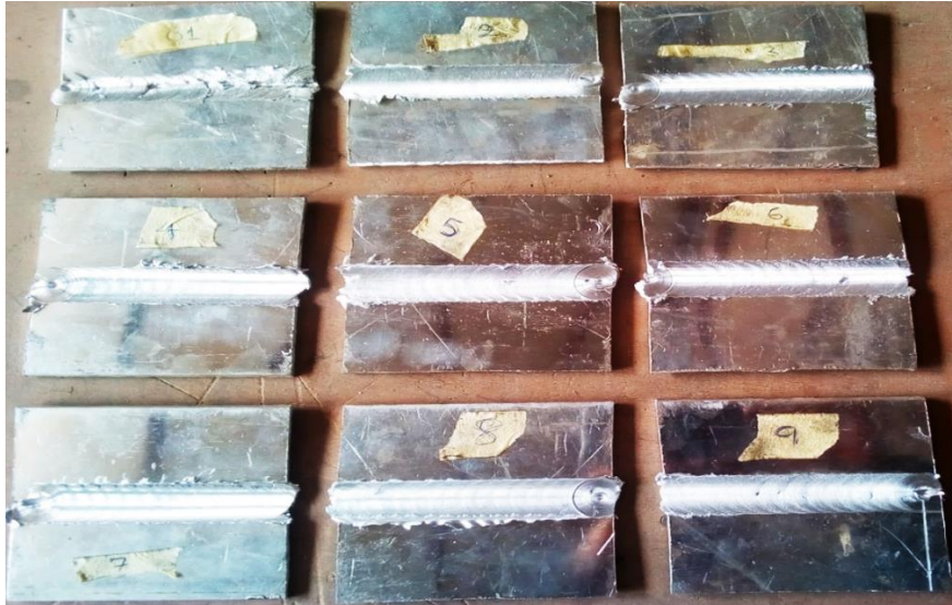
Figure 6: The friction stir welded joints produced using the developed MFS
