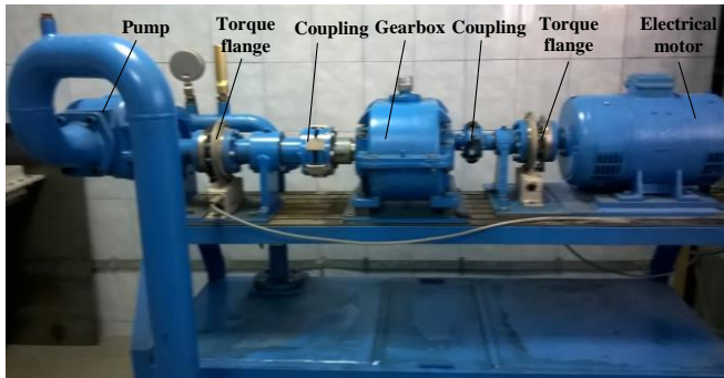
Figure 1. Main components of the test stand [13]
