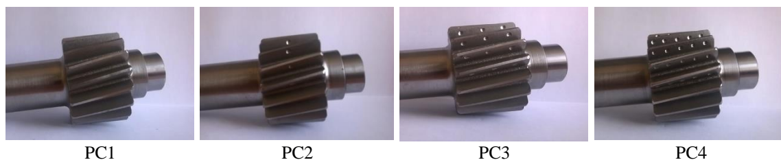
Figure 2. Pinions with different failure status
