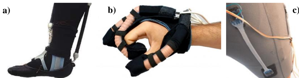
Figure 4: Wearable soft robotic devices. a) ankle rehabilitation with soft actuator [27], b) soft robotic glove [28], c) soft sensing suit [29]
