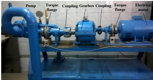
Figure 1. Main components of the test stand [13]
