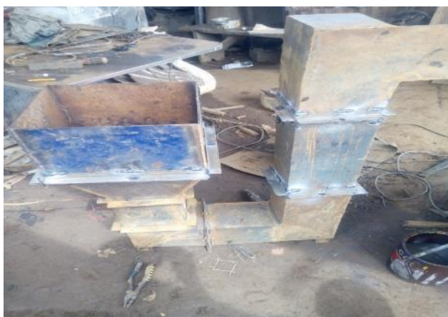
Figure 8: Fabrication of the Iron Ore Sintering System.
