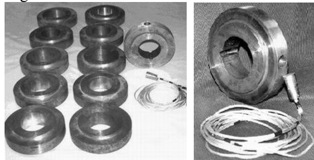
Figure 2 Assembly of conical pin fitted Pt-Pt/RH thermocouplings
