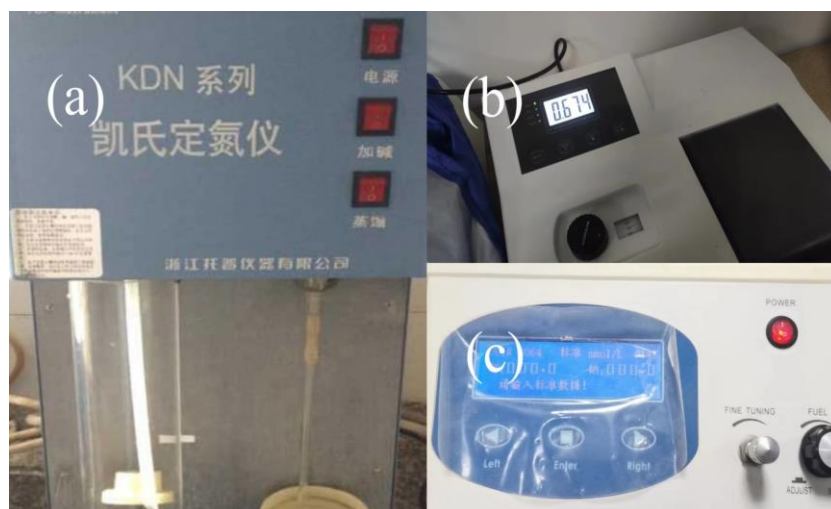
Figure 2. (a) KDN-08C Kjeldahl nitrogen analyzer (b) 722N Spectrophotometer (c) FP6410 Flame spectrophotometer
