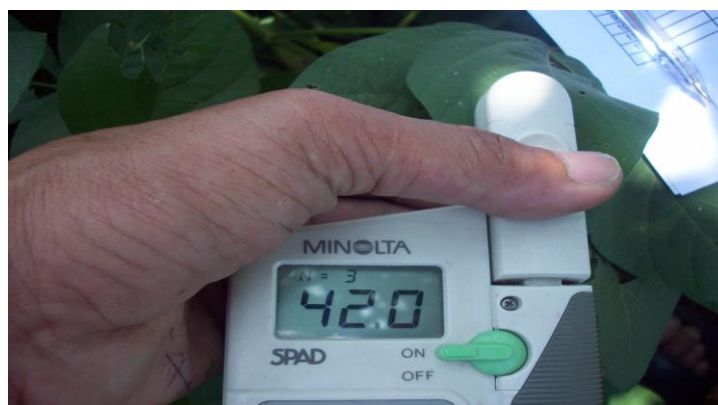
Figure 1. Measurement of leaf chlorophyll index using a SPAD digital chlorophyllmeter
