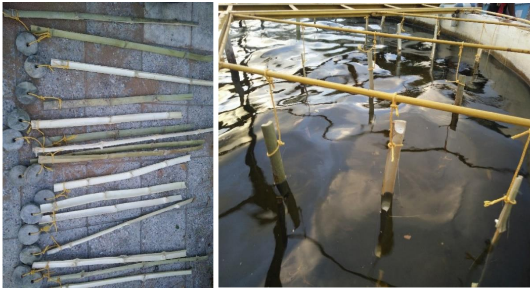
Figure 1. Fabricated split bamboos and their erection in 13 ton circular tanks
