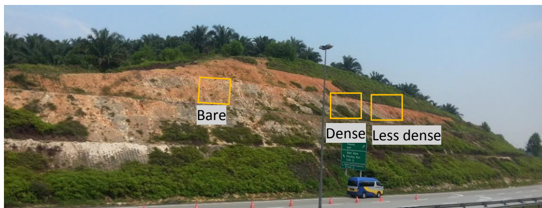
Figure 2. Experimental plots located on the third berm of the slope. From the left: bare plot (B), dense plot (D), and less dense plot (LD)
