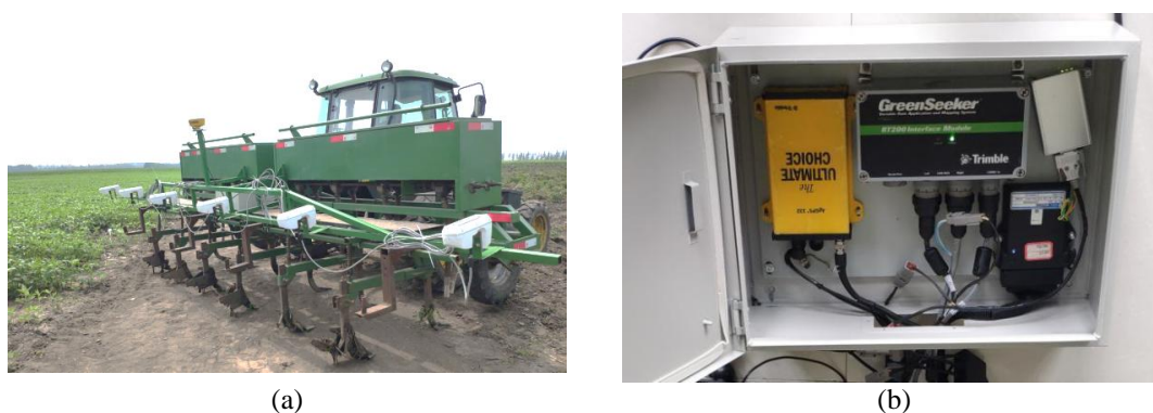
Figure 2. Ground-based remote sensing detection platform for the acquisition of soybean canopy NDVI data. (a) Data acquisition site; (b) Interior of the remote sensing platform control box
