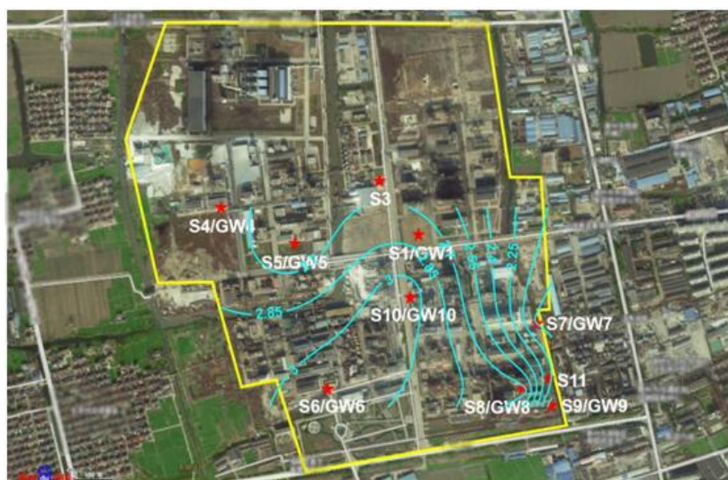
Figure 1. Groundwater flow direction of the contaminated site
