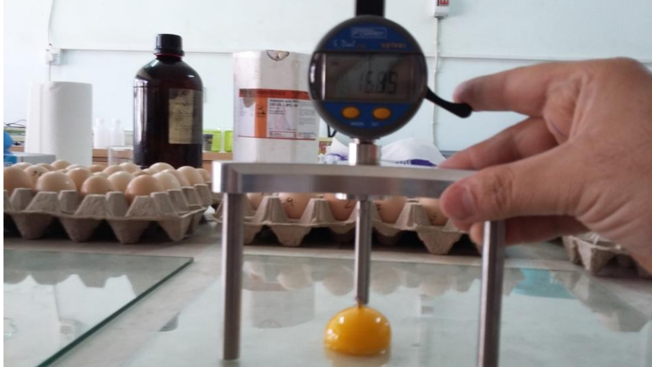
Figure 5. Spherometer used for measure yolk height
