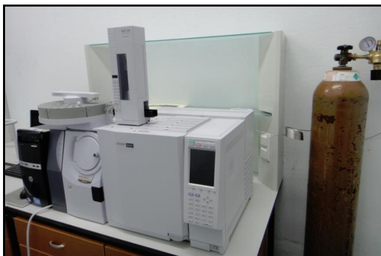
Figure 2. Shimadzu QP 2010 Plus GS-MS system for chromatography analyses of volatiles
