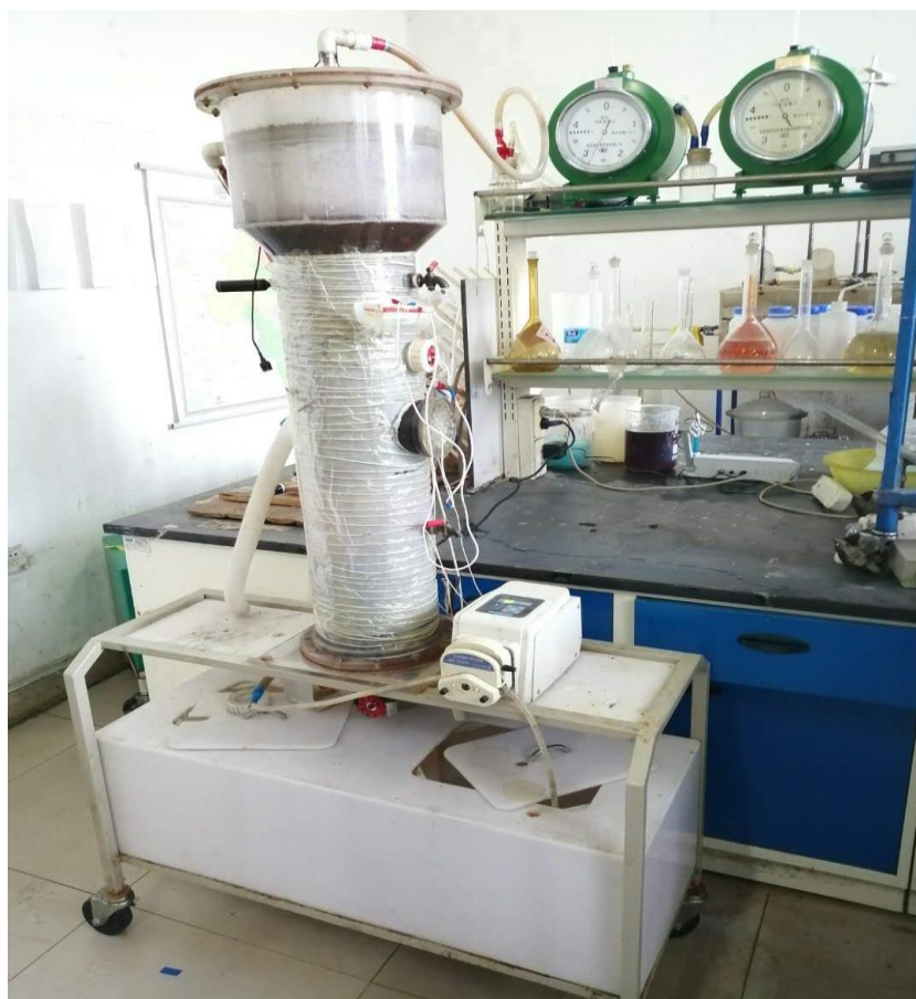
Figure 2. Physical photo of the UASB reactor
