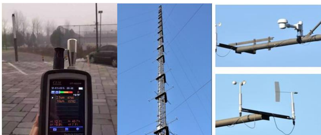
Figure 7. The near-surface test equipment 1.5 m away from the ground and meteorological observation iron tower
