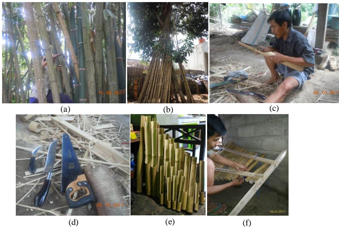
Figure 4. The angklung paglak manufacturing: Bamboo logging, done by the maker using saw and buding (a); Bamboo drying, the culm (alive bamboo) is air dried without being exposed to direct sunlight in upright position (b); Harmonizing angklung tones use ladeng lanang (a knife usually use by Using men), done by shaving the bamboo tube to get the right tone according to its potential (c); traditional tool used to manufacture angklung ( ladeng lanang to shave the bamboo tube, buding to cut bamboo's branch, saw to log and cut the bamboo into pieces) (d); a set of angklung paglak tubes as the result of angklung harmonizing (e); and the arrangement of angklung tubes using plastic rope at the wood buttress (f)
