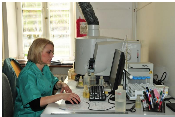
Figure 3. iCAP 6500 duo Thermo Scientific ICP–OES instrument used for determination of analysed chemical elements. (Photo: I. Jaroń)
