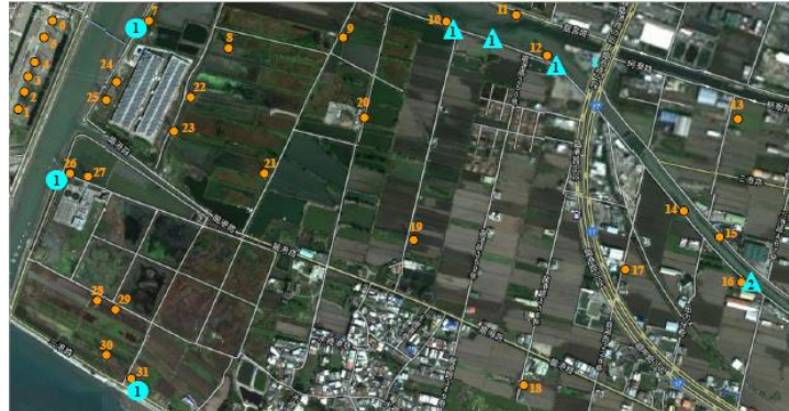
Figure 36. The distribution map of bird carcasses around the transmission towers where the symbols ● and ▲ stand for the survey results in Stage 2 and Stage 3, respectively. The numbers inside the symbols are the counts of the bird carcasses.
