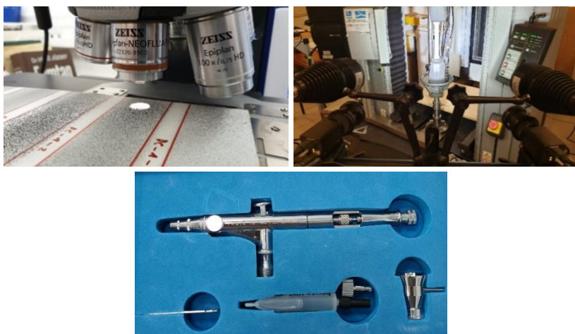
Figure 5. Zeiss Optical Stereo Microscope (a) and ARAMIS 5M test setup with tensile testing machine (b) and Iwata AirBrush pistol (c)
