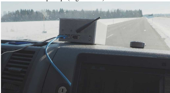
Fig. 3. Testing vehicle passing by the RSU, seen on the left side of the road. The OBU can be seen on top of the dashboard next to the external GPS receiver (on the right). Information about the data transferred during the tests is instantly seen on the laptop screen.
