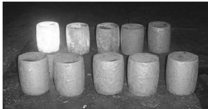
Figure 8. Forged parts of the upsetting experiment
