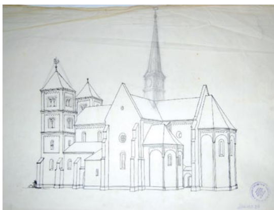
Figure 6. Another plan for the restoration of Calvinist Church in Ócsa: sketch of a crossing tower and heightening of towers, around 1922 [5]
