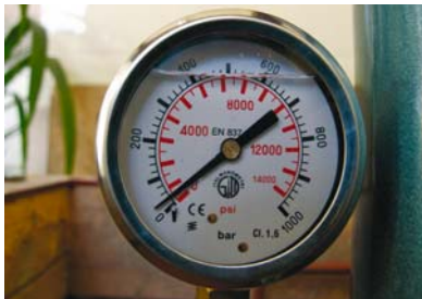
(e) the vertical stress measuring gauges
