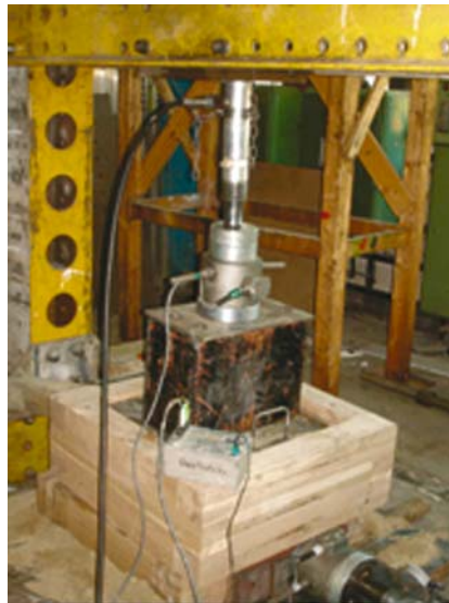
Figure 8. Direct shear test for waste (after [7])
