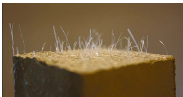
Figure 10. The broken surface of 40x40x160 mm test piece
