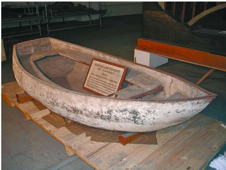
Figure 1. Joseph-Louis Lambot's boat made of reinforced concrete in 1855 [3]
