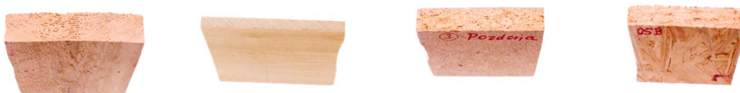
Figure 2. Photos of samples from left to right: PWB, MPB, PBC, OSB
