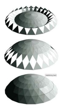
Figure 4 Schema of the of the pantadome erection
