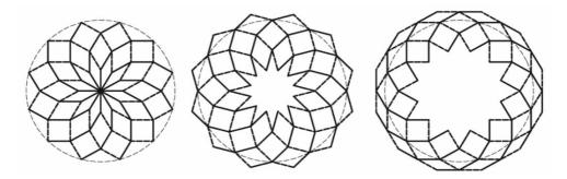
Figure 8: Deployable sequence of a ring structure developed by Z. You and S. Pellegrino
