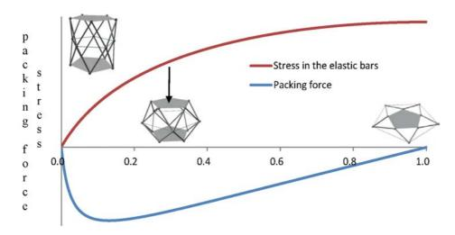
Figure 14 Packing (downward) force in function of the relative displacement of the top nodes and tensile stresses in the elastic, pentagonal bars (0 corresponds to the deployed and 1 to the packed, planar state)
