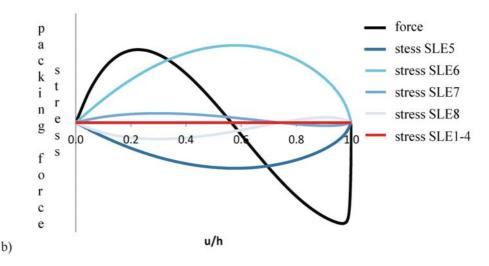
Figure 12 Packing simulation of a self-locking pantographic structure: basic simulated element (a); characteristic of the packing forces and the resulting stresses in the scissors in function of the relative displacement of the center node (0 corresponds to the deployed and 1 to the packed, planar state) (b)
