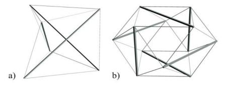
Figure 1: Examples for tensegrity units: a) the tensegrity tripod b) expanded octahedron
