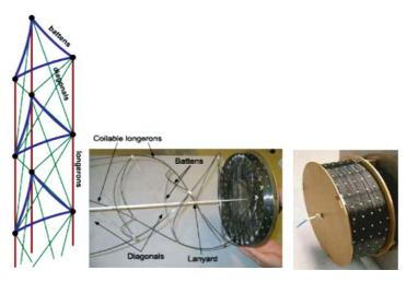
Figure 16 Coilable mast by the Jet Propulsion Laboratory
