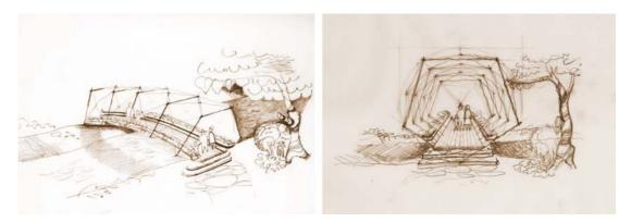
Figure 15 Bridge design applying the deployable pentagonal antiprismatic system [5]
