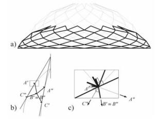
Figure 7 Iris dome designed by Hoberman : schematic model (a), complex hinge system (b, c) [35]
