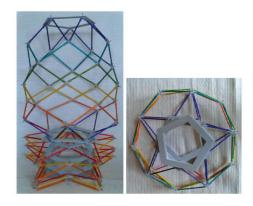
Figure 17 Physical model of antiprismatic pop-up mast by the authors (deployed and packed configurations) [5]
