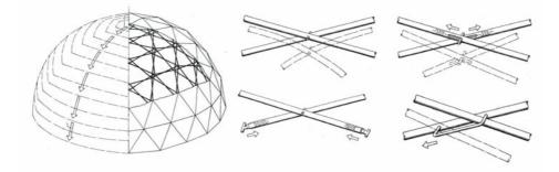
Figure 11 Zeigler's patent for collapsible self-supporting structure: dome and scissor details [45]
