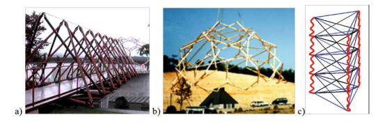
Figure 3 Foldable bridge (a) and deployable dome (b) by ATAKE Space Design Lab. Co. in the Hanamizuki Park, Japan `96 [20]; schematic drawing of the deployable mast controlled by active and passive cables by the former Deployable Structures Laboratory (c) (passive cables with red lines, active cables with blue lines, scissors with black)
