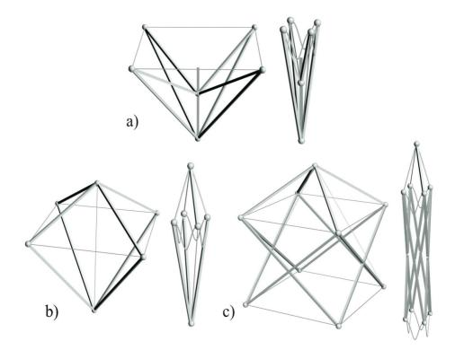
Figure 5 Post-stabilized cable-strut deployable structural units by Liew and Krishnapillai
