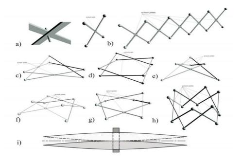
Figure 2 A simple scissor joint and the basic element, one SLE (a); the lazy tong (b) and some secondary basic units of scissor-like deployable structures (basic units with symmetrical scissors (c, d), pyramid type units (e, f) skew type units (g, h)); bent scissor elements (i)
