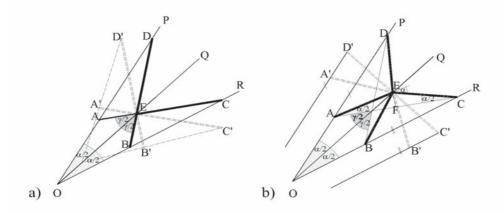
Figure 6 (a) Classic SLE and (b) the simple angulated element (illustrated in accordance with [32])
