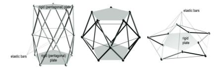
Figure 13 Basic segment and its packing sequent of antiprismatic pop-up mast proposed by Hegedűs
