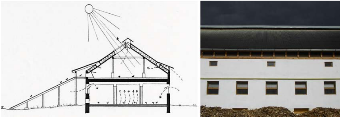
Figure 34-35 Converted two-storied shed with a granary attic in the bio chicken-farm in Tornyiszentmiklós with side and ridge ventilation (architects: Dr. Gábor Reischl, Zoltán Laczó)
