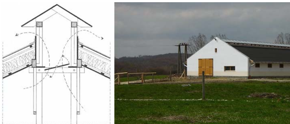
Figure 32-33 Heightened ridge ventilator in a fowl-house in the bio chicken-farm in Tornyiszentmiklós (architects: Dr. Gábor Reischl, Zoltán Laczó)
