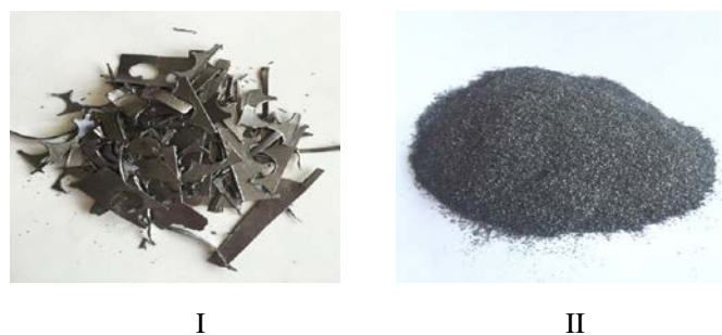
Figure 1. Graphite foil wastes (I) and pGFW (II).
