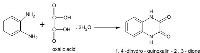
Scheme 1. Preparation of 1,4-dihydroquinoxalin-2,3-dione
