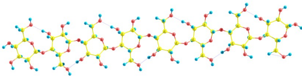
Figure 7. Optimized structure of cellulose (8 glucose units) which is optimized at PM3 semi-empirical quantum mechanical method. COOH is replaced with OH of CH 2 OH.
