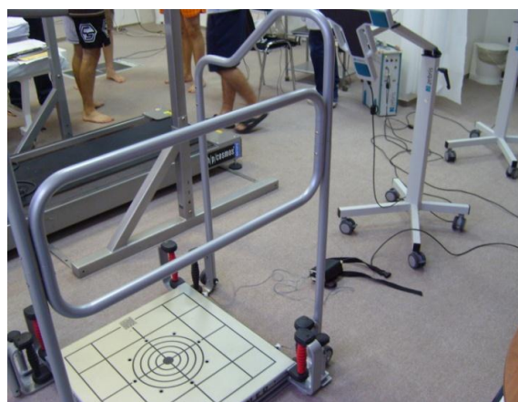
Figure 2. Measurement arrangement. PosturoMed plate secured by springs of identical strength in different directions. Ultrasound-based measuring head located to the side of the object at 30 degrees.
