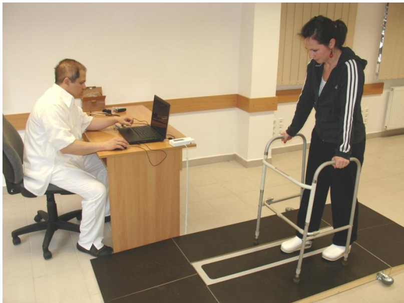
Figure 8. Calibration of force transducer shoes on the scale platform
