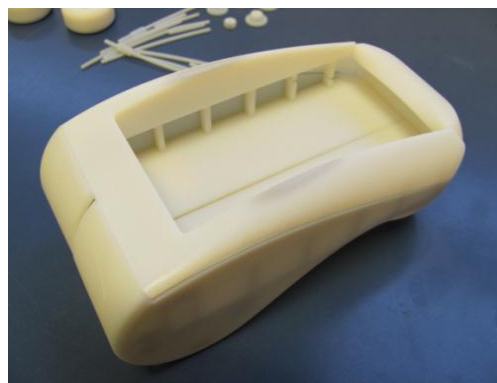
Figure 4. 3D printed docking equipment
