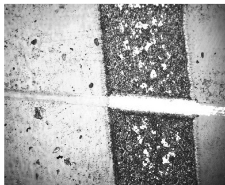
Fig. 6. Typical scratch track line through silver thin films and copper filaments
