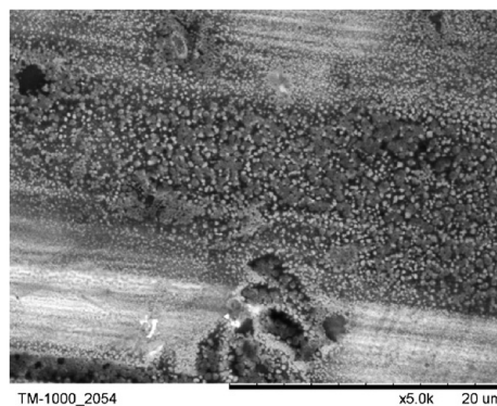
Fig. 4. Typical defects on surface of copper filaments
