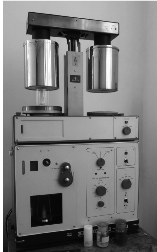
1. ábra A derivatográf Fig. 1. The Derivatograph
