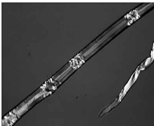
Fig. 1. Spruce latewood fibre showing dislocations in pol. light
