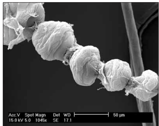
Spruce fibre balloon swelling in phosphoric acid [6,7].
